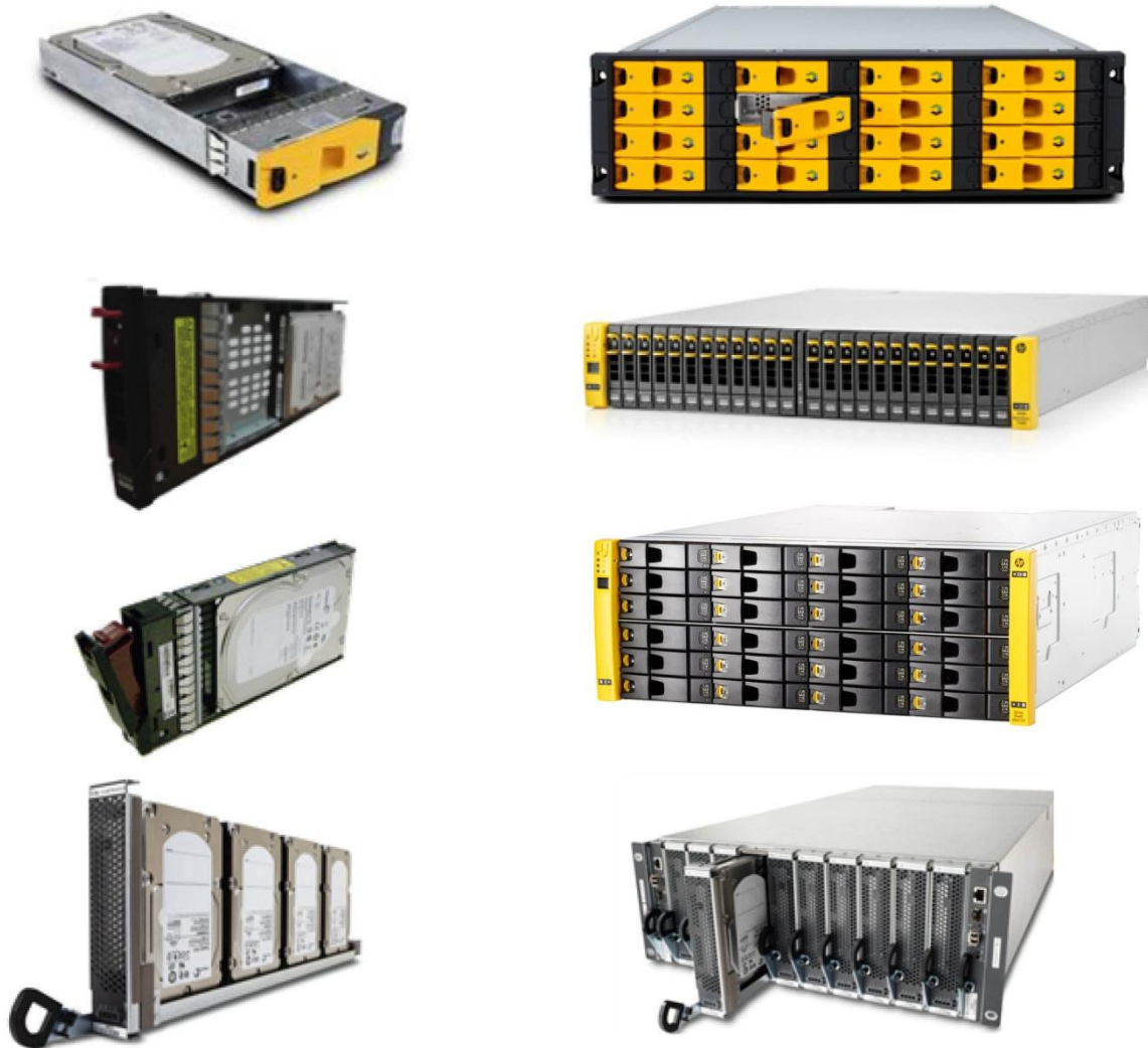
Figure 4. From top to bottom: a Drive Magazine and a Drive Chassis for the HP 3PAR StoreServ F-Class, HP 3PAR StoreServ 7200 Small Form Factor (SFF, 2½"), HP 3PAR StoreServ 7200 Large Form Factor (LFF, 3½"), and HP 3PAR StoreServ 10000
