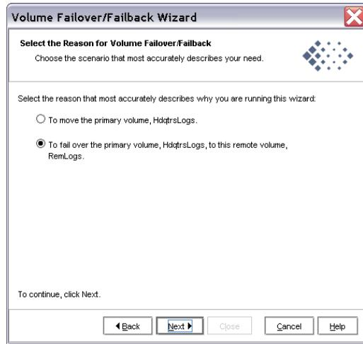
Figure 2.25. Selecting to failover to a remote volume
