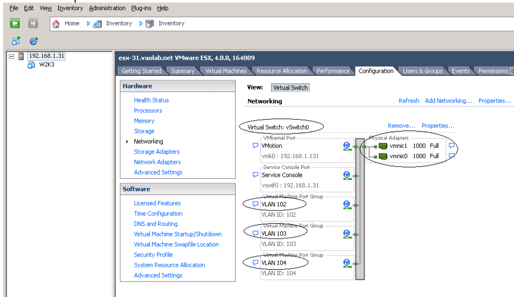
Figure 1-76 Both NICs for Profile ESX-1 are connected to the network through Multiple Networks, VLANs are configured as Port Groups within the virtual switch.
