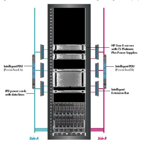
Figure 3: The iPDU communicates with each server's iLO Management Engine before you power on the servers.
