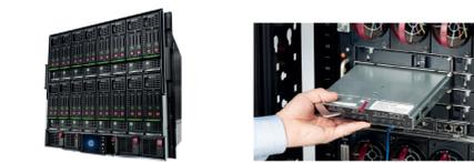
The new HP BladeSystem c7000 Platinum enclosure delivers the **highest performance** including the fastest connectivity with 56 GB FDR InfiniBand, 40 GB Ethernet for high performance, low-latency networking and 16 Gb Fibre Channel ready with superior scalability for storage.
